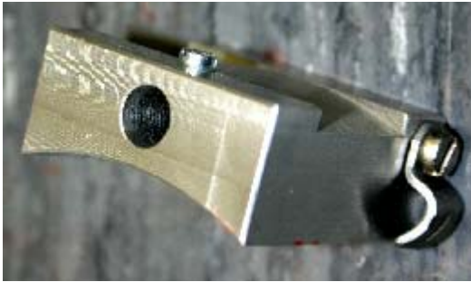
Picture 4 (The temperature sensor holder)
