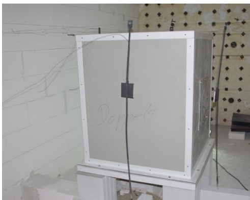
Valve Fire Shelter before start of test
