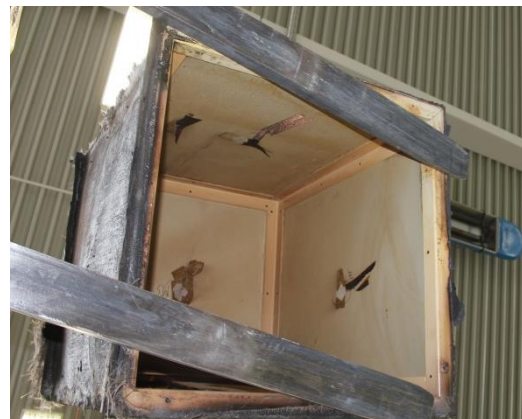
Valve Fire Shelter Internally after >60min. at 1200°C/2000°F
