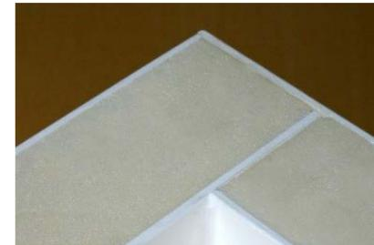
The sandwich construction of polyurethane foam between an inner and outer layer of glass-fiber reinforced polyester sheeting provides superior means of constructing a HOT BOX. It combines very low thermal conductivity with great strength and a high resistance to wear and corrosion.
