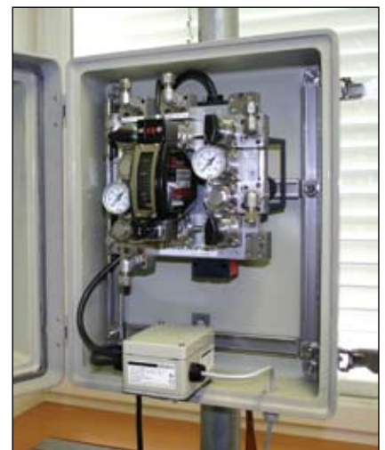
Fig. 1: A typical hot box - a well-insulated enclosure made from glass reinforced polyester with a smart conduction heater (behind substrate). In this case housing an analytical sample conditioning system built using a Parker Hannifin Intraflow SP76-compatible modular substrate.
