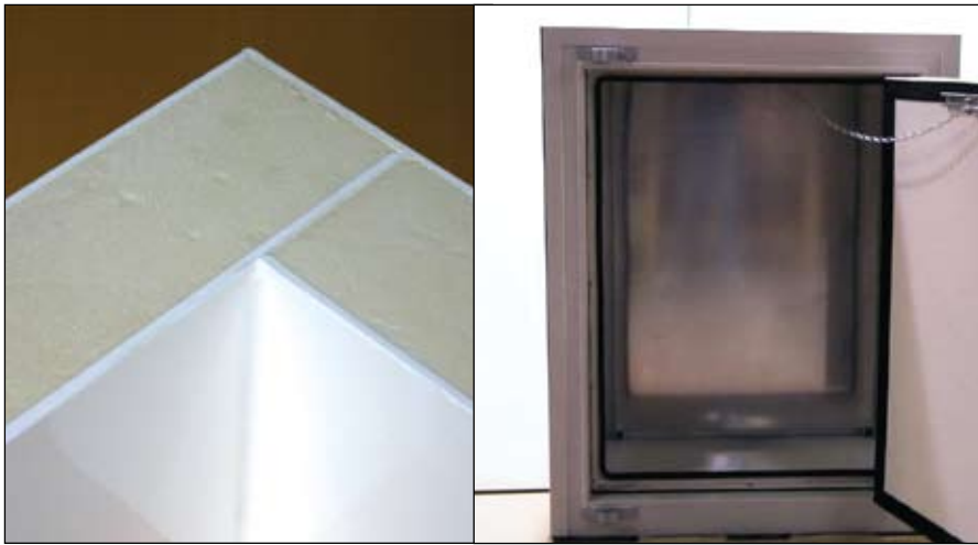
Fig. 3: Left: The sandwich construction principle using GRP sheeting and an insulation layer. Right: Typical finished hot box with 100 mm of PUR foam insulation, for use in extreme climates such as the Arctic.
