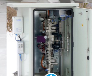
Compact field enclosure with three separate analyzers and sample conditioning (from Astute).
